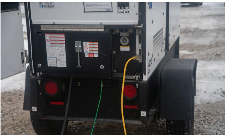
Connection of 3 phase electrical wires into portable generator
