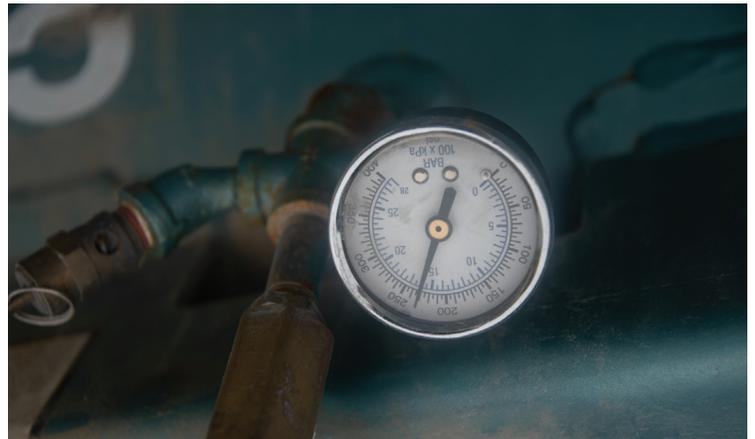
Pressure gauge on air compressor tank
