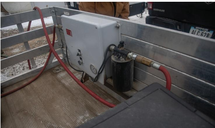
Air compressor hose 1, coming into the oiling box and on the right, hose 2 coming from the oiling box to the captive bolt gun
