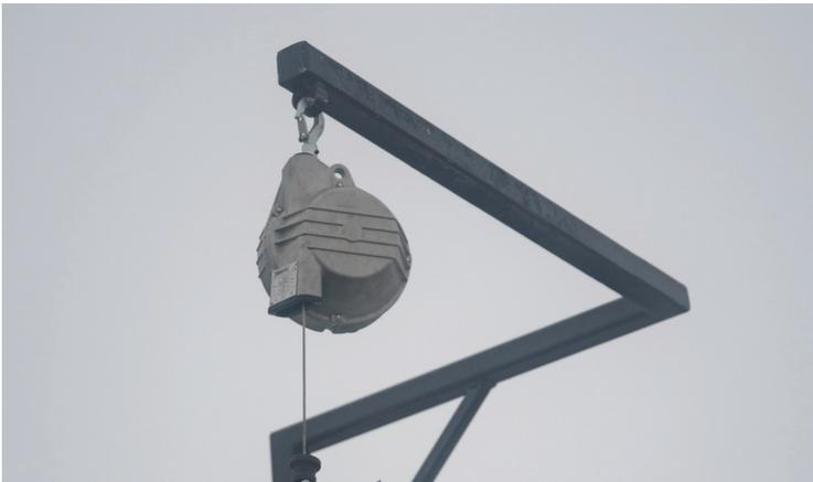
Counter balance attached to the counter balance stand
